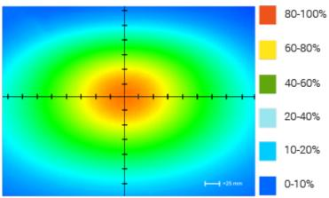
Optical measurement taken using AL126-WHIIC Rev. A @ 200 mm
