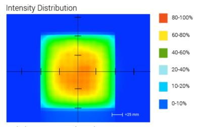
Optical measurement taken using BL128-WHIIC
