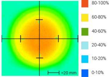
Optical measurement taken using DF196-100WHII3 @ 25mm
