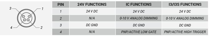
The functions listed above are only applicable when this product is configured with built-in 24V, IC, I3, or I3S control, with an A-coded 4-position Male M8 connector.
