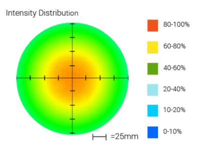
Optical measurement taken using DF198-180WHII3 @ 100mm
