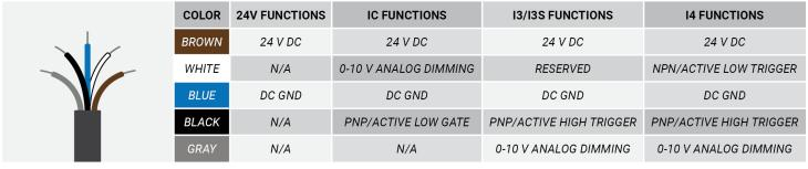
The functions listed above are applicable when this product is configured with built-in 24V, IC, I3, I3S, or I4 control, without the optional A-coded 5-position Male M12 or A-coded 4-position Male M8 connector.
