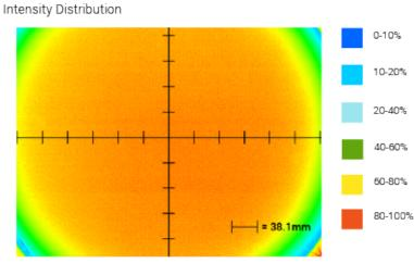
Optical measurement taken using DL080-WHIIC @ 25mm
