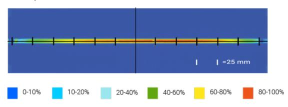
Optical measurement taken using DL15112-WHIIC @ 25mm
