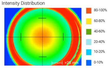
Optical measurement taken using DL2230-62513 @ 25 mm
