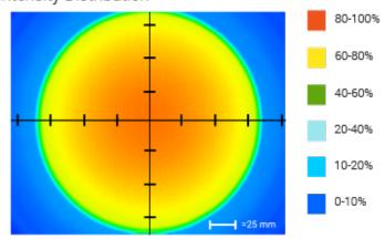
Optical measurement taken using FX0808-WHII3 @ 200mm
