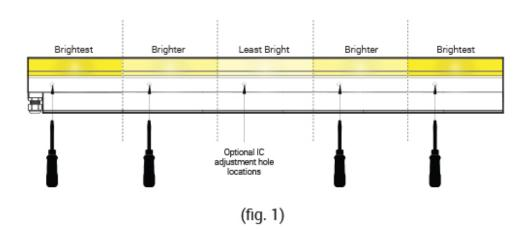
Controlling each 6" (152mm) section independently and making the center of the line less bright and the outside of the immediate camera viewing radius brighter ultimately results in better imaging.
