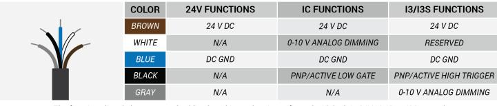
The functions listed above are applicable when this product is configured with built-in 24V, IC, I3, or I3S control, without the optional A-coded 5-position Male M12 or A-coded 4-position Male M8 connector.
