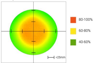
Optical measurement taken using RL36120-625200XLIC @ 300 mm
