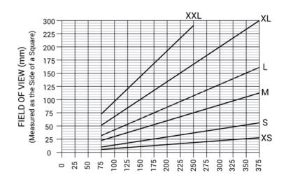
STAND OFF FROM OBJECT TO LIGHT HEAD (mm) Indentify desired FOV and stand off, then specify nearest illuminated area size
