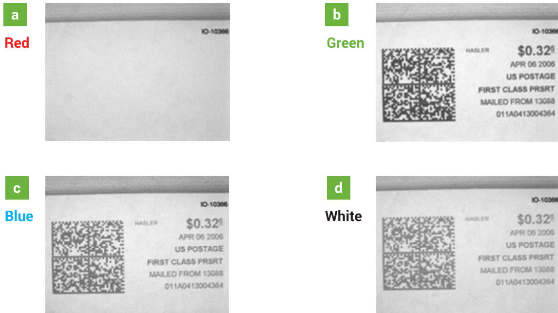
Fig. 35: a – Red mail stamp imaged under Red light, b - Green light, c - Blue light, generating less contrast than green, d – White light, generating more contrast than either Blue or Green light. White light will contrast all colors, but it may be a contrast compromise.
