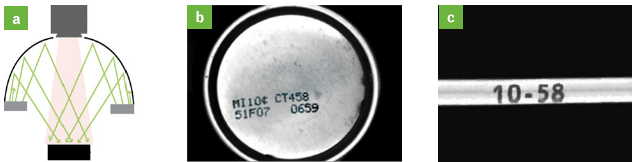
Fig. 23: a - Diffuse dome light function diagram, b - Bottom of a concave soda can illustrating even illumination across the surface, enabling a read of the printing, c - Glass rod, character reading.
