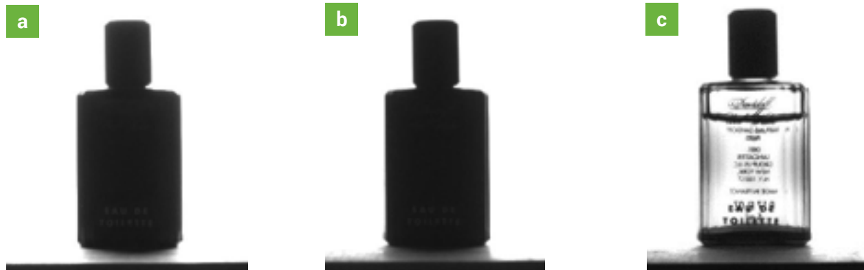
Fig. 42: Bottle fill level inspection with back lighting, a - 660 nm red, b - 880 nm IR, c - 470 nm blue.
