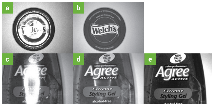
Fig. 62: A change in “lighting – object – camera” geometry or type may be more effective than applying polarizers to stop glare, a – Coaxial Ring Light w/o Polarizers, b – Coaxial Ring Light w/ Polarizers (note: 2 ½ f-stop opening), c – Coaxial Ring Light w/o Polarizers, d – Coaxial Ring Light w/ Polarizers (note some residual glare), e – Off-axis (light optic axis parallel to the object long axis)
