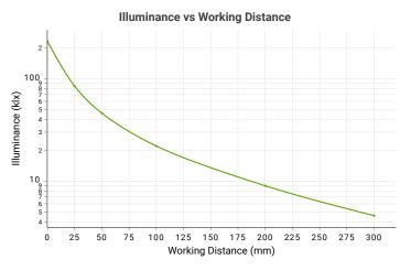
Linear Backlights, while typically oriented behind the object of interest, can also be used for highly diffuse front illumination at short to medium working distances. The chart to the left shows the BL313's intensity as it's distance from the inspection surface changes.
