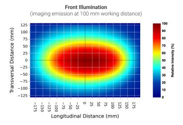
Both intensity distribution images shown above have been taken using a 12-inch white BL313 unit (BL31312-WHIIC).
