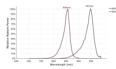
Near-infrared (NIR) imaging is a machine vision technique using longer wavelengths of 700-1000 nm to penetrate specific materials that are otherwise opaque to under the visible spectrum. When paired with a NIR camera, a NIR light can be ideal for applications such as fill level inspection, circuit board inspection, food safety inspection, and medical imaging.
