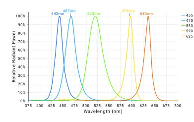
Visible color illumination consists of using wavelengths between 400-700 nm to either create or eliminate contrast on an inspection subject based on differences in a features color hue. When referring to a color wheel, simply remember the following: like colors reflect and brighten surfaces; conversely, opposing colors absorb and darken surfaces.
