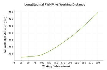
Both Full Width Half Maximum (FWHM) vs Working Distance plots shown above have been measured using a 12-inch white BL313 unit (BL31312-WHIIC).
